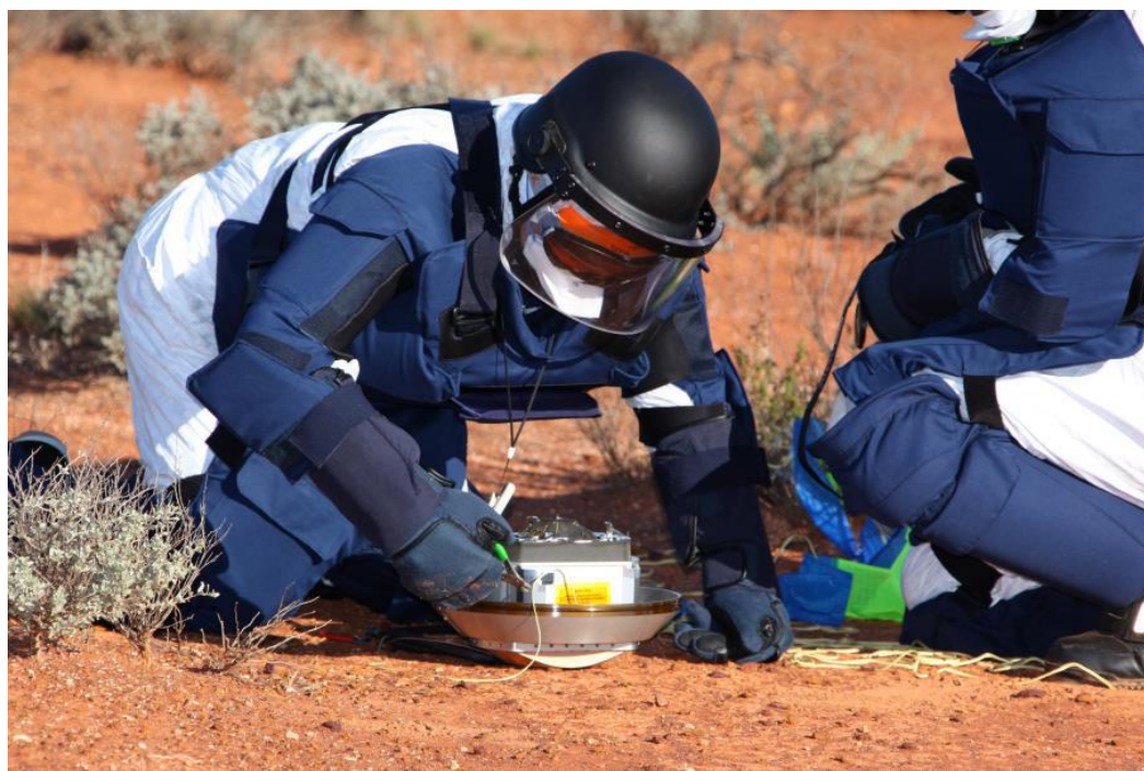
Figure 5. Hayabusa return capsule safing of batteries (Image credit: JAXA)
