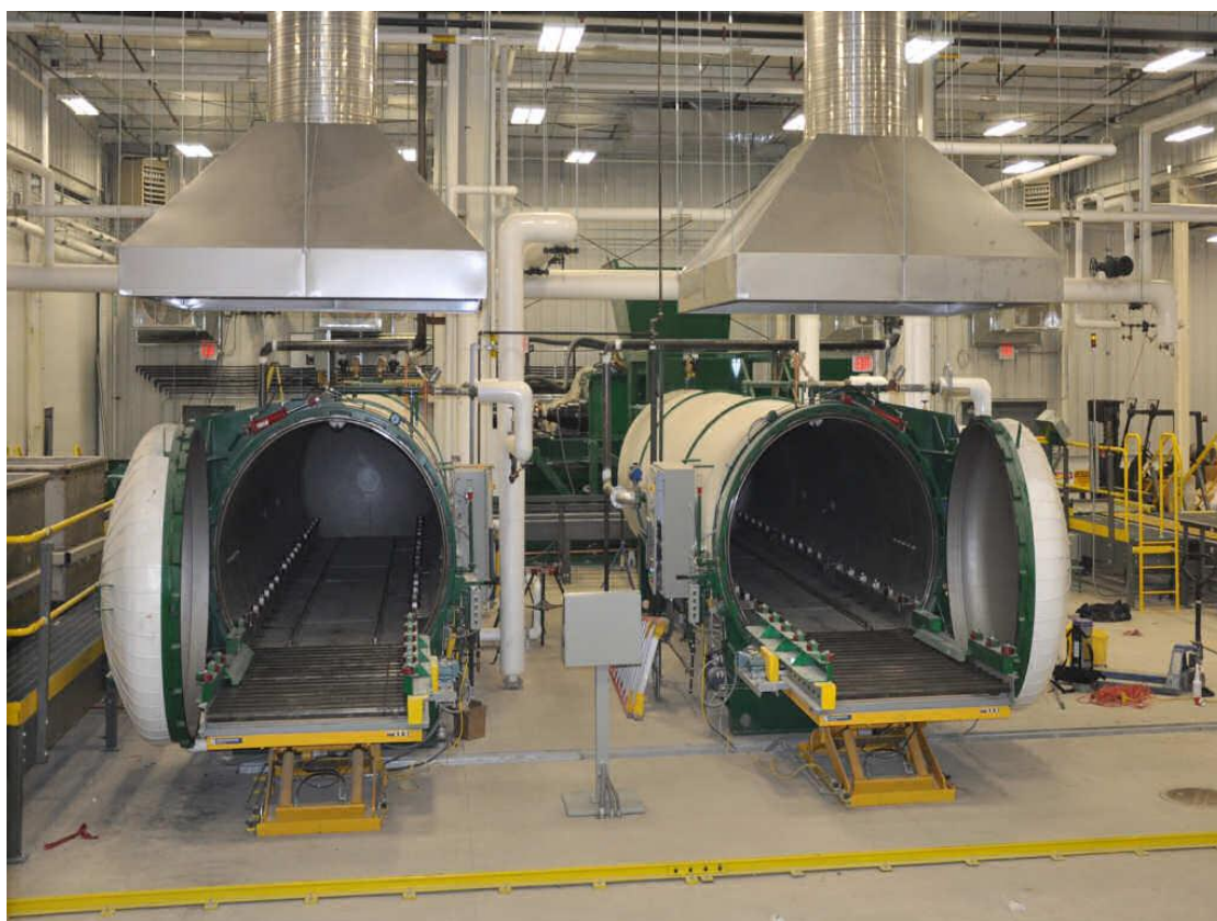
Figure 12 shows large medical waste autoclaves. Note the rollers to allow access of large containers. Image credit Bondtech Corporation, www.medicalwasteautoclaves.com
